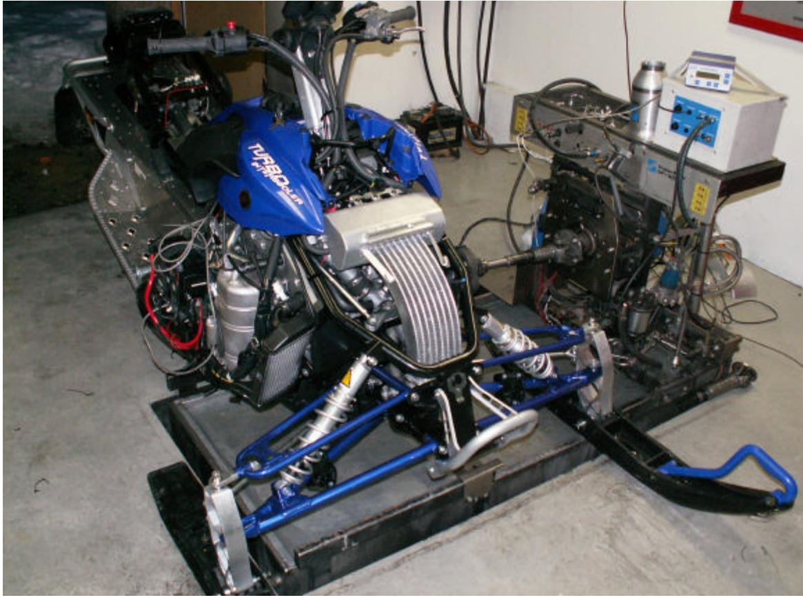
The higher power requires a new setup in the clutch. We have tested and designed new clutch weights specially for turbo use to both the Phazer, Apex, RX1, RS, and RS Viking. We make the new weights in house with our CNC-machines.
