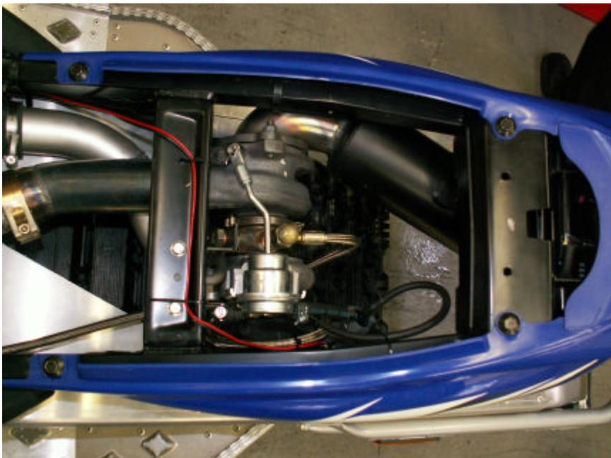
The turbo and muffler is located under the seat. The weight is about the same as the stock muffler.
