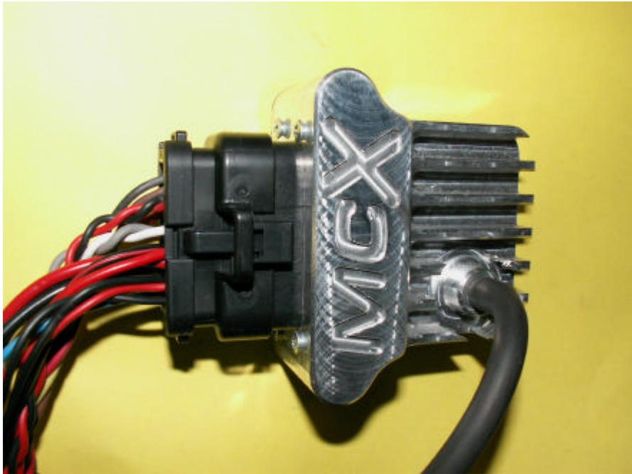
This new system can not only deliver the exact amount of fuel at any load, temperature and altitude, but also control the turbo pressure. When you go up in altitude, the EFI-box automatically rises the turbo pressure to retain the power.
